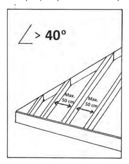
For use on a roof with a slope of more than 40 degrees, a waterproof membrane is not necessary. The distance between the roofbeams may not exceed 50 centimeter.
