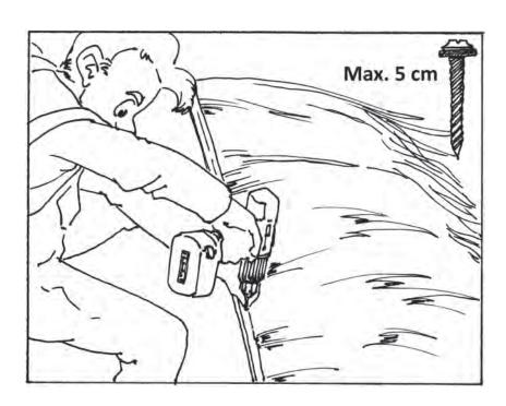
Attach the shinglerails using special screws with rubber washers with a maximum length of 5 centimeter.
