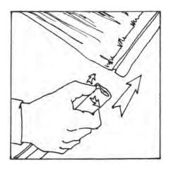
Open the plastic rail just enough that it is possible to slide in a single shinglesheet.
