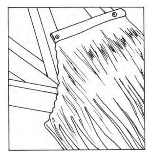
First prepare a rail so that it easily can cover the distance between the cornerbeam and the next one. slide a piece of rail over the shingle and fold it as if you're preparing a normal shinglerail. Cut the piece that is not covered by the rail in a curve (See illustration).
