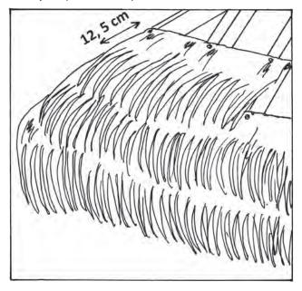
Now work your way up, row by row, staggering the shingles as you go. (Start one row with a full shingle, the second with a half-shingle, the third with a full shingle, and so on.) Place ervery next row of shingles at 12,5 centimer distance from the previous one.
