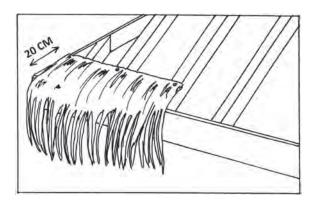
You place the prepared rails of shinglesheets directly on the roofbeams.
