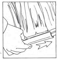
Fold the rail over the Shingle sheet until it becomes stuck. Now you're ready to attach the shinglerail to the roof.
