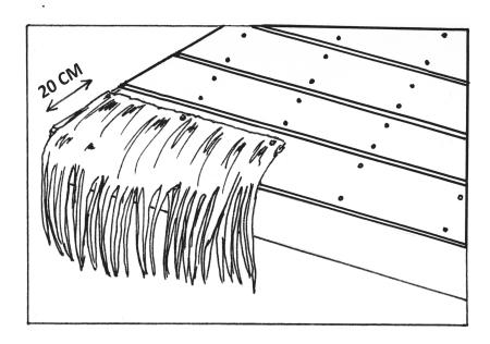
The first shinglerail is placed at 20 centimeter from the roofedge.
