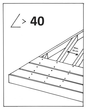
Place planks over the entire roofsurface and attach them firmly to the roofbeams. The distance between the roofbeams may not exceed 50 centimeter.
