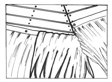
Finally place a third shingle that is prepared in the usual manner and fold it over the corner so that it covers the two previously placed shingles. Attach this sheet to the beams with screws with rubber washers.
