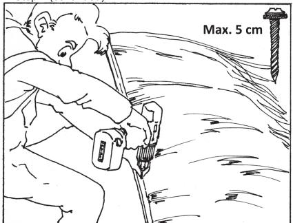
Attach the shinglesheets using special screws with rubber washers with a maximum length of 5 centimeter.
